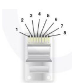
RJ45 connector pin assignment
